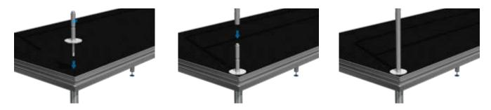
To mount the handrails on top of the stage a special adaptor is needed. This adapter is mounted through the deck in the corner side where the little dot (cap) can be removed. As the dot is removed the adaptor fits in a special leg which offers the needed support for the adapter to hold the handrails. The handrail just can be put on the pivot holder.
