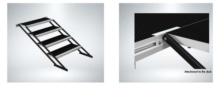
Adjustable stairs ensure quick and smooth assembly. They are made of heavy-duty steel sections and the stairssteps are filled with antislip plywood. The staircase is self angled because of the movable steps mounted in the frame.
